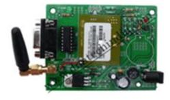
This is a plug and play GSM Modem with a simple to interface serial interface. Use it to send SMS, make and receive calls, and do other GSM operations by controlling it through simple AT commands from micro controllers and computers. It uses the highly popular SIM300 module for all its operations. It comes with a standard RS232 interface which can be used to easily interface the modem to micro controllers and computers.
