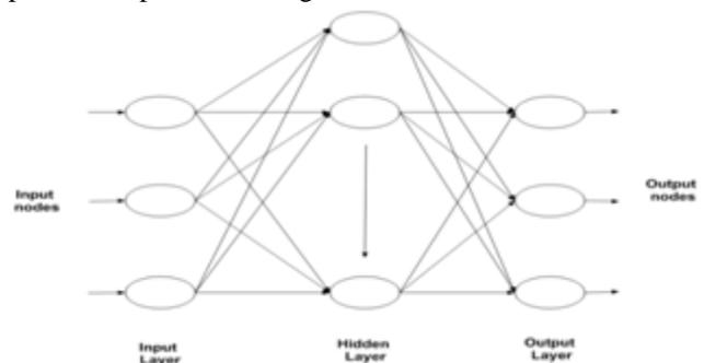
Fig architecture of artificial neural network
