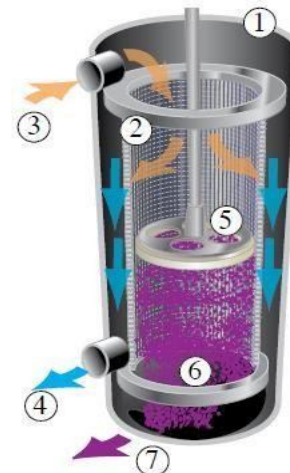
Fig 6. Eaton DCF filter. 1) Filter housing, 2) Filtermedia, 3) Inlet, 4) Outlet, 5) Cleaning disc, 6) Debris 7) Drain outlet [4].
