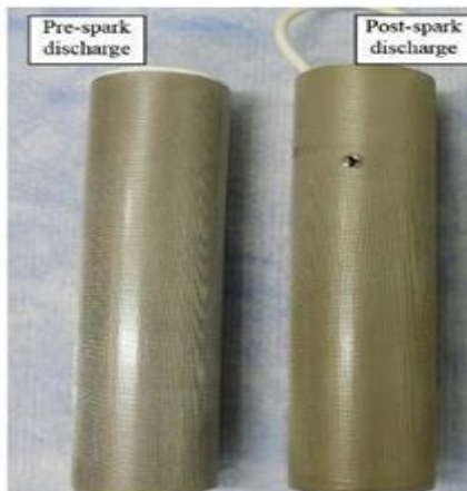
Fig 2. Filter damage due to cathodic hotspot [1] .
