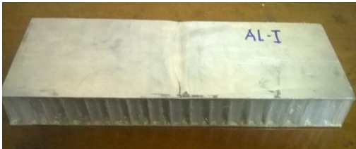
Fig.8. Specimen AL-I of Aluminium (A3003 H19) – Polypropylene panel after bending
