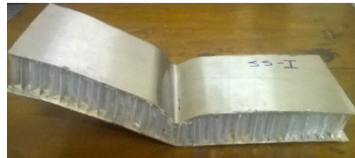
Fig.2. Specimen SS-I of Stainless Steel – Polypropylene panel after bending
