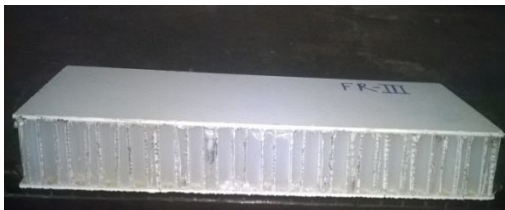
Fig.18. Specimen FR-III of GFRP – Polypropylene panel after bending
