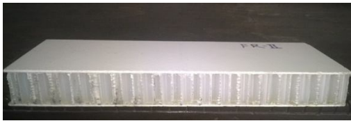
Fig.16. Specimen FR-II of GFRP – Polypropylene panel after bending
