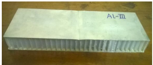
Fig.12. Specimen AL-III of Aluminium (A3003 H19) – Polypropylene panel after bending
