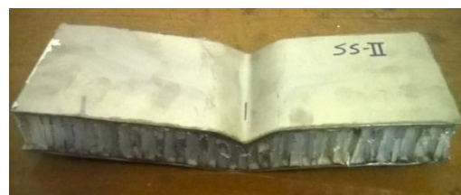
Fig.4. Specimen SS-II of Stainless Steel – Polypropylene panel after bending
