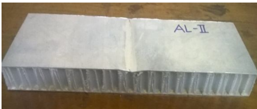
Fig.10. Specimen AL-II of Aluminium (A3003 H19) – Polypropylene panel after bending
