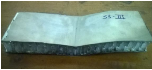
Fig.6. Specimen SS-III of Stainless Steel – Polypropylene panel after bending
