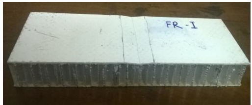
Fig.14. Specimen FR-I of GFRP – Polypropylene panel after bending
