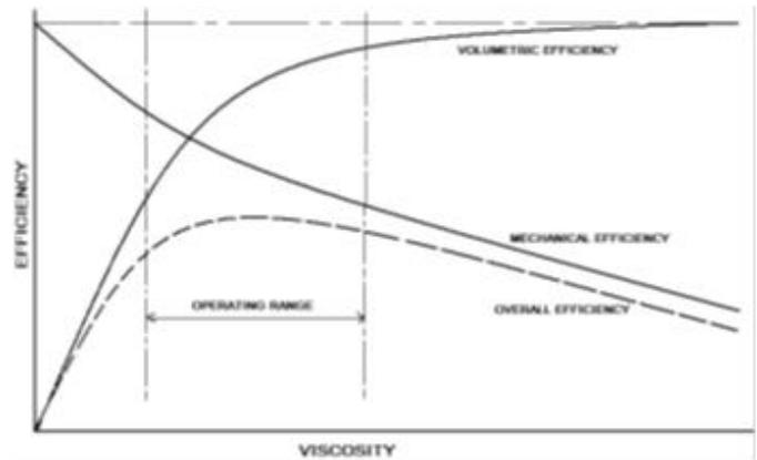
Graph 1: Efficiency v/s Viscosity (Hydraulic Fluid Properties and its influence on system performance)
