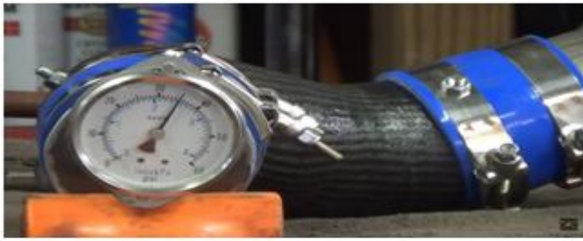
Fig no.4 Pressure test on carbon fibre composite showing max value of 38psi.
