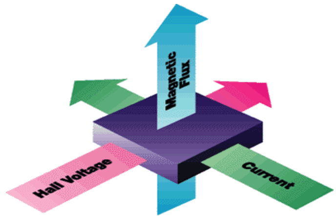
Fig 2: Principle of Hall Effect sensor
