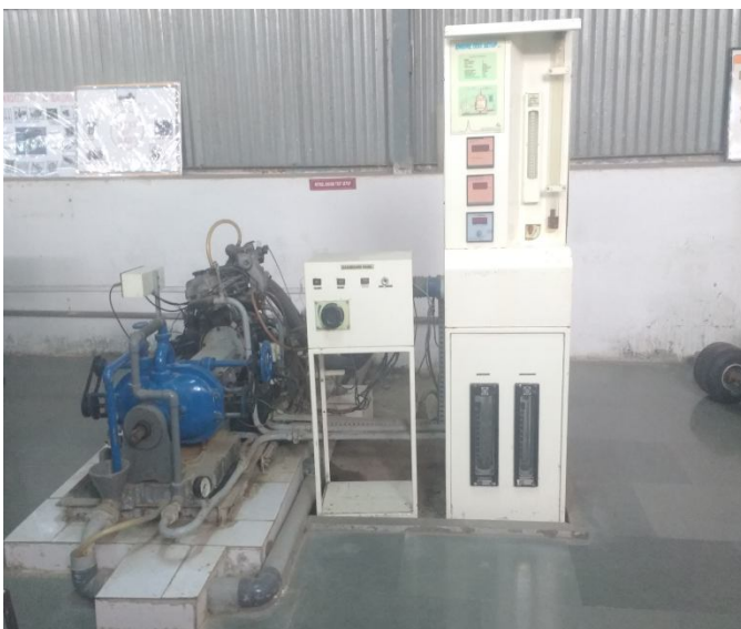
Fig 2. Photographic view of 3 cylinder 4 stroke SI engine
