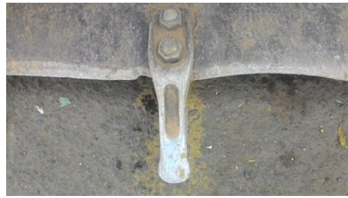
Fig.4. Abrasive wear on surface of bucket tooth.
