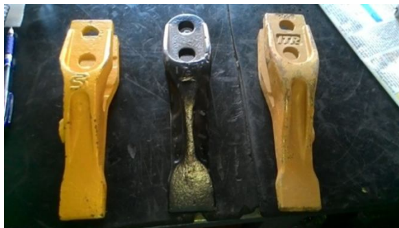
Fig.3. New bucket teeth
