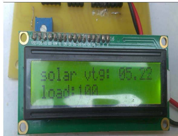
d) Above Img. shows when solar voltage is less than 6.12V
