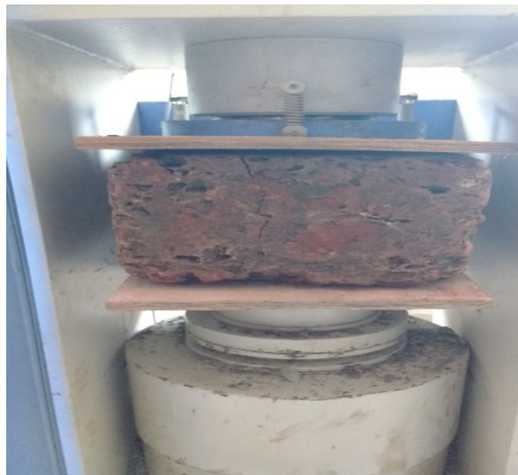
Compression testing of Konkan laterite
