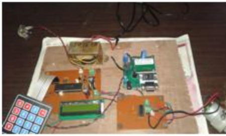
Fig.4 Prototype of Bank Locker Security System
