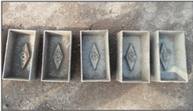
Fig. 2 Dies used for making bricks
