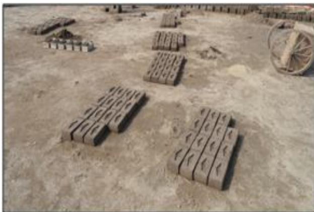
Fig. 3 Drying raw bricks before baking
