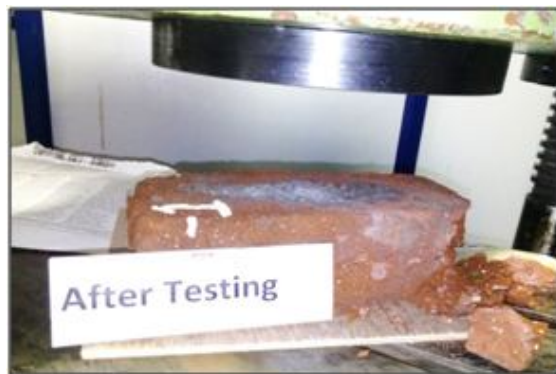
Fig. 7 Specimen of sample 1 after compression test
