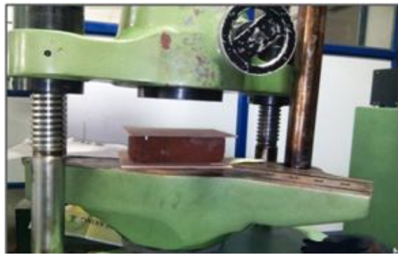
Fig. 6 Specimen of sample 1 during compression test
