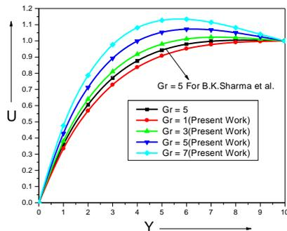
Fig.2 Transient velocity profiles for different Gr
