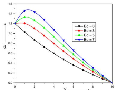
Fig. 8 Temperature profiles for Ec variation
