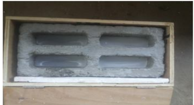
Fig 2: concrete block with paraffin wax
