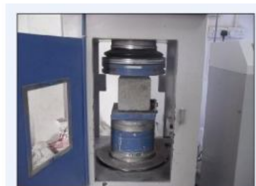
Fig: Compressive Strength Test
