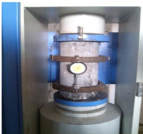
Fig: specimen set up to find stress strain behavior
