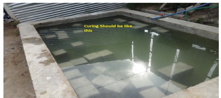
Fig: curing cubes
