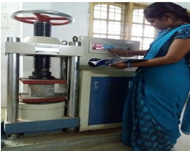
Figure.4. Testing of compressive strength of specimen
