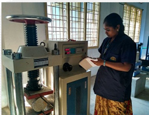
Figure.5. Testing of split tensile strength of specimen
