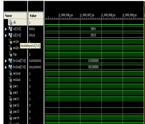
Fig8: Output waveforms for Multi field packet classification with parity
