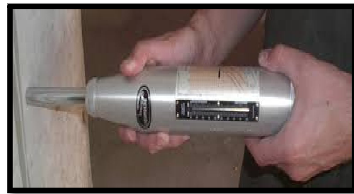
Fig.7 Rebound hammer test
