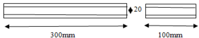
Fig 4 Sandwich material beam dimensions
