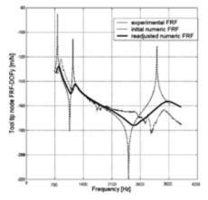
Fig. . Experimental, initial and readjusted FRF.
