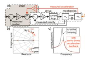
Fig. 2. Vibration damping by velocity set point acceleration feedback: Control diagram, (b) velocity loop root locus and (c) tool tip compliance
