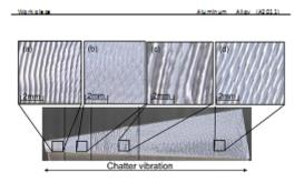
Fig.1. Machined surface after milling test.
