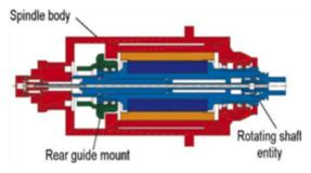
Fig. 4. The HSM spindle bearing system.
