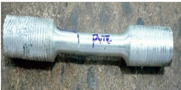
Fig 5: Tensile test specimen of pure aluminum 6061
