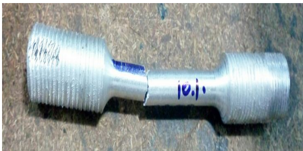
Fig 7: tensile test specimen of Al 6061 with 6% sic and 10% fly ash
