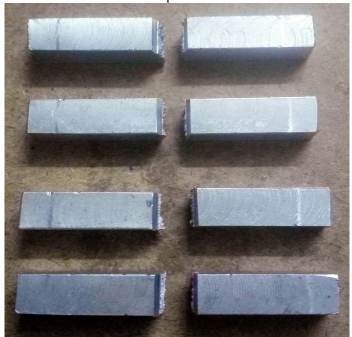
Fig 10: impact test specimens of Al 6061 with fly ash and sic all compositions (0%, 5,3%, 10,6%, 15,8)
