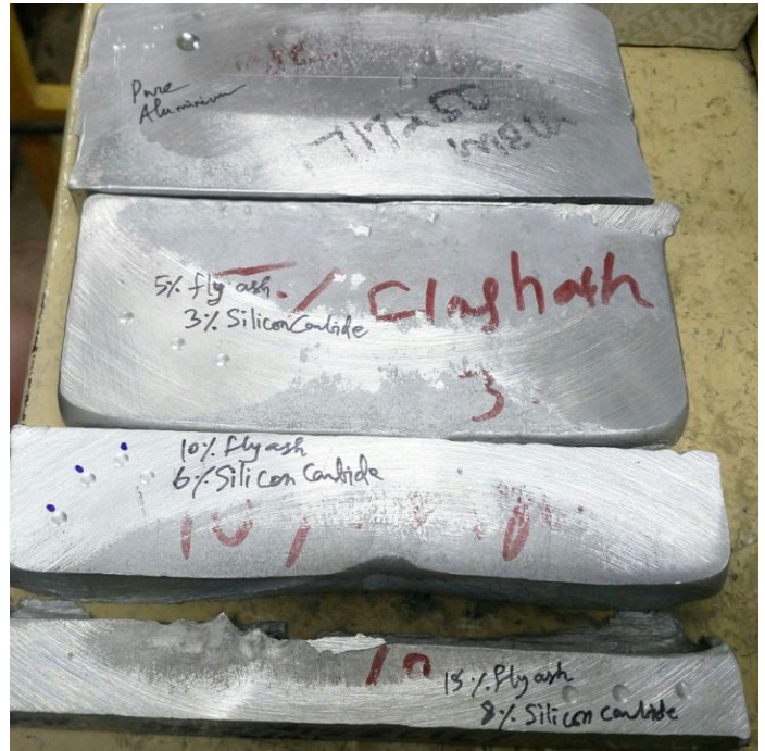
Fig 9: Hardness test specimens of Al 6061 with fly ash and sic all compositions
