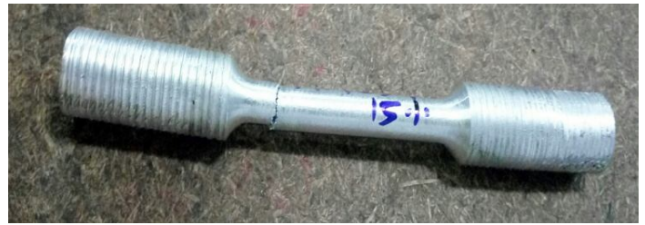
Fig 8: tensile test specimen of Al 6061 with 8% sic and 15% fly ash
