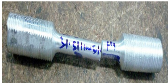
Fig 6: tensile test specimen of Al 6061 with 3% sic and 5% fly ash
