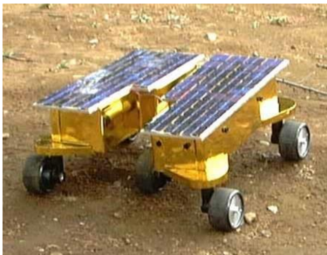
Figure 8.2. Development model of a lunar rover for the Japanese mission SELENE-II.
