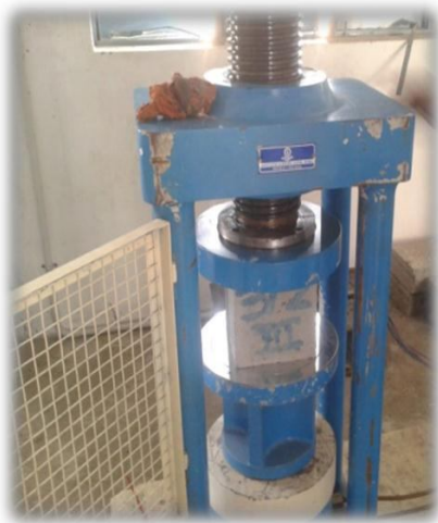
Fig 1: Compressive Strength Test
