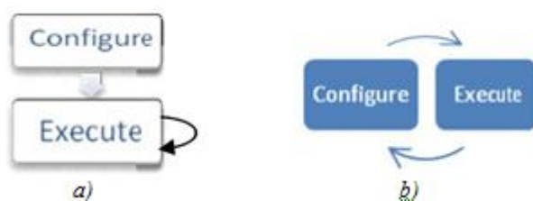
Fig. 11.a) Principle of static reconfiguration b) Principle of dynamic reconfiguration.
