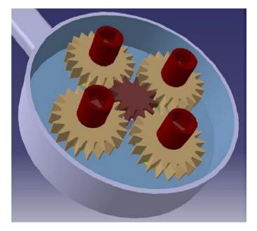
tow truck and available nearest mechanic to solve the problem. This always happen to the elderly or female drivers. Based on the capability of torque application by these drivers, a vehicle all-wheel-nuts remover is designed. The remover is designed to be ergonomic to be used, easy maintenance, easy storage, easy to handle and able to remove all nuts at once.
