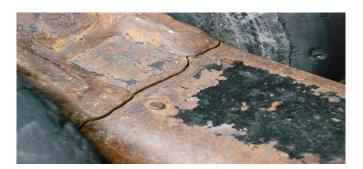
Front axle beam takes about 30-40 % of total vehicle weight. The main three reasons of failure of mechanical components are Corrosion, wear and fatigue. Main reason for failure of front axle beam is the fatigue damage due to continuous fluctuating loads which acts from irregular road surface. Therefore, the research on the fatigue life of different vehicle parts has important value.
