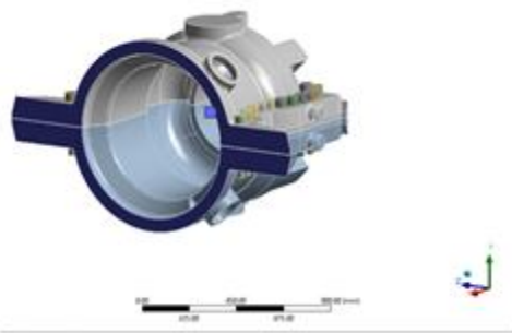
Fig.2: Boundary Condition for casing
