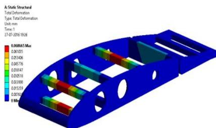
Figure 5.7: Total deformation wing box without Honeycomb Structure
