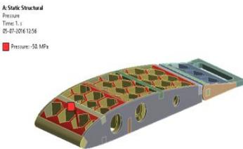
Figure 4.8: Tension loads on wing box with honeycomb structure
