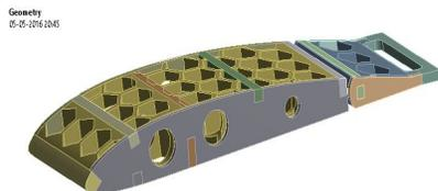
Figure 4.2: Three dimensional model of wing box with honeycomb structure
