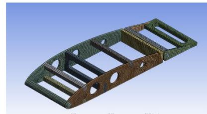
Figure 4.3: Meshed wing box model without honeycomb structure
