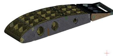
Figure 4.4: Meshed model wing box with honeycomb structure
