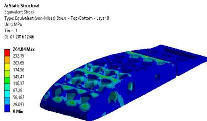
Figure 5.6: Equivalent Stresses Wing Box with Honeycomb Structure
