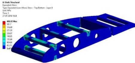
Figure 5.5: Equivalent Stresses Wing Box without Honeycomb Structure
