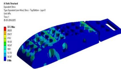
Figure 5.2: Equivalent stresses of wing box with honeycomb structure
