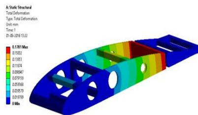
Figure 5.3: Total deformations wing box without Honeycomb
