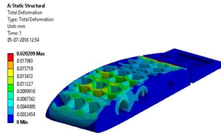
Figure 5.8: Total deformations wing box with Honeycomb Structure
