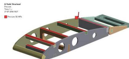
Figure 4.5: Compressive loads on wing box without honeycomb structure
