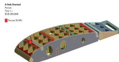
Figure 4.6: Compressive loads on wing box with honeycomb structure
