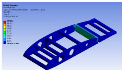
Figure 5.1: Equivalent stresses of wing box without honeycomb structure
