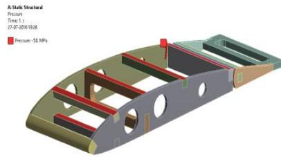
Figure 4.7: Tension loads on wing box without honeycomb structure
