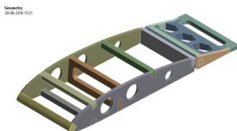
Figure 4.1: Three dimensional model of wing box without honeycomb structure
