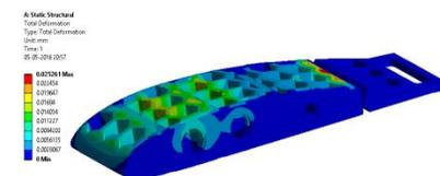
Figure 5.4: Total deformations wing box with Honeycomb structure
