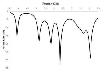
Fig-2 Return Loss of Patch 1
