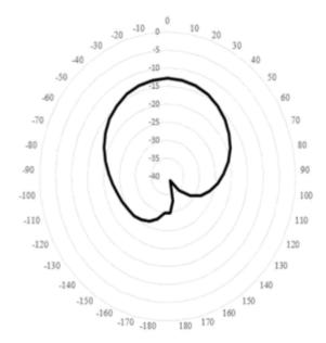
Fig-6 Radiation Pattern at  $4.8~\mathrm{GHz}$
