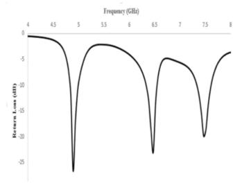
Fig-4 Return Loss of Patch 4
