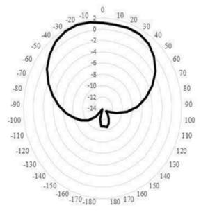
Fig-9 Radiation Pattern at 7.4 GHz
