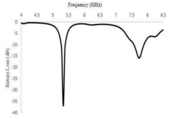
Fig-3 Return Loss of Patch
