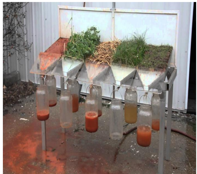
Fig 1. Collection of water sample by using rainfall simulator method (Source: University of Delaware)
