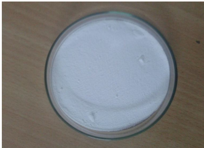
Fig-KOH supported on alumina catalyst used for transesterification reaction.
