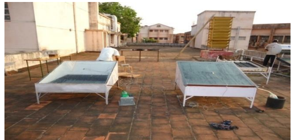
Fig. 3 photographic view of Experimental set up of Solar stills with basin area of 1 m 2
