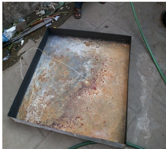
Fig.12 Photographic view of Galvanised Iron basin material after degrad
