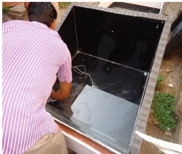
Fig.10 Photographic view of after removing the scale on toughened glass basin material of Solar Still
