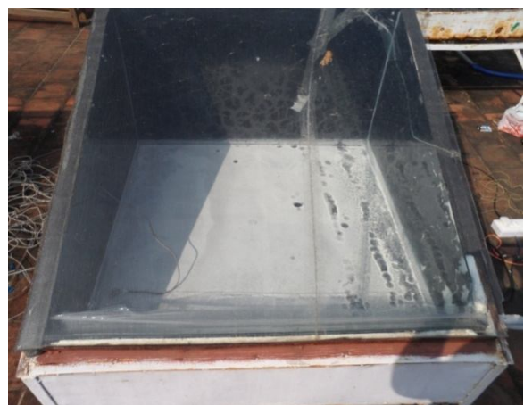
Fig. 9 Photographic view of scaling on toughened glass basin material of Solar Still
