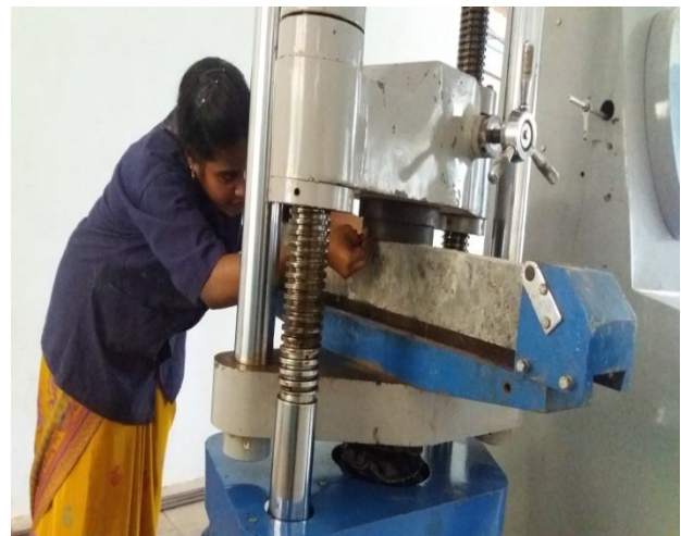
FIG.4 Testing of flexural strength of specimen
