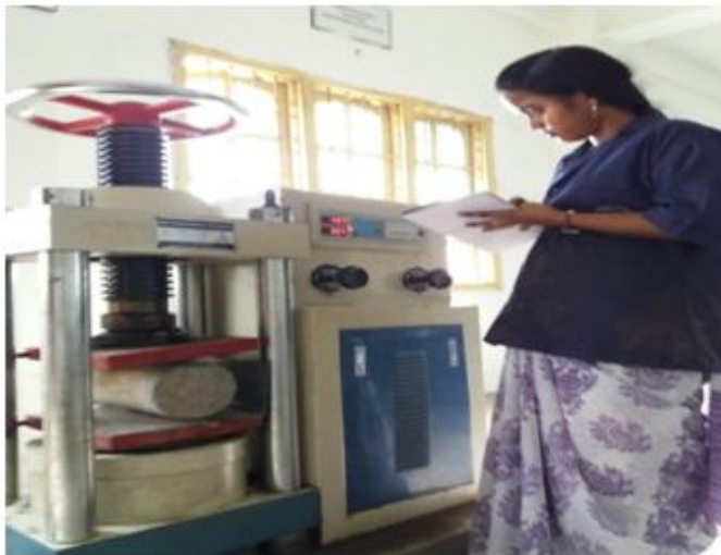
Figure 3 Testing of split tensile strength of specimen
