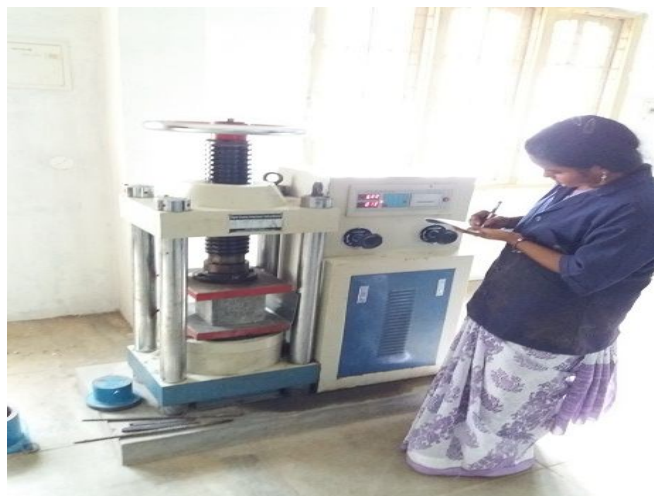
Figure.2.Testing of Compressive strength of specimen
