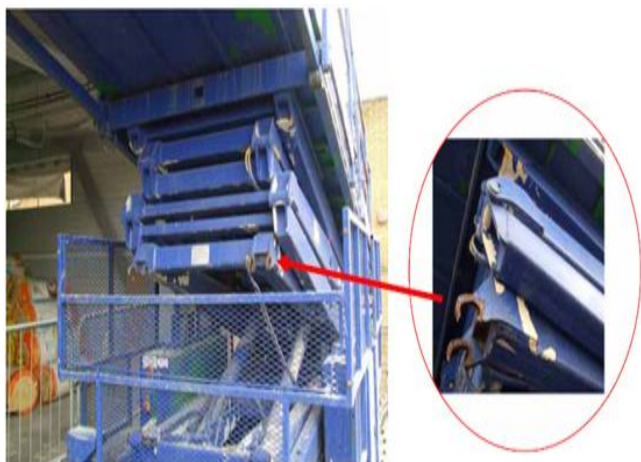
Fig: Failure of Hydraulic Scissor lift due to maximum deformations
