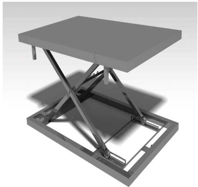
Fig: CAD model of Hydraulic Scissor lift
