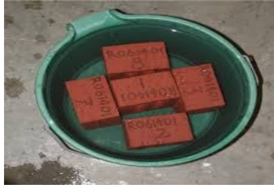
Plate 1 Bricks soaked in water for Water Absorption test
