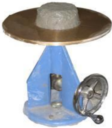
Plate 2. Flow Table test
