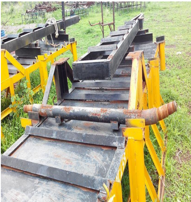
Fig. 3 Bending of sugarcane trolley axle
