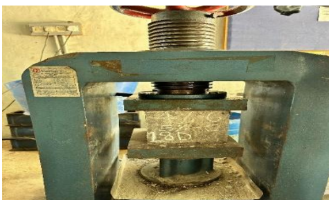
Fig -10: 4% admixture & 5% coral shell powder 28 days
