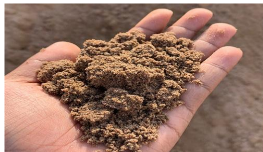
Fig – 3: Fine aggregate
