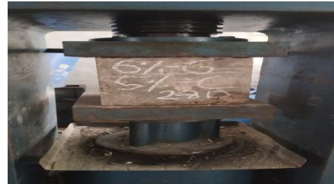
Fig -12: 6% admixture & 5% coral shell powder 28 days
