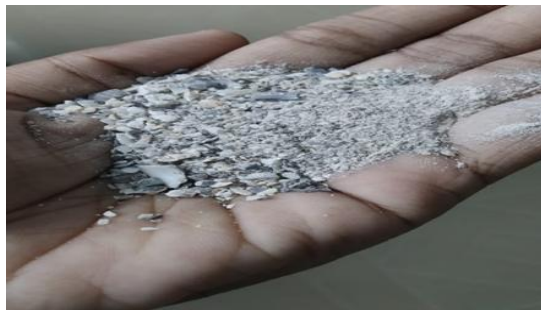
Fig –4: Oyster shell powder
