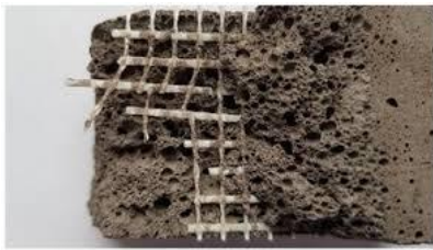
Figure no. 3 Glass Fiber Reinforcement in Geopolymer Concrete
