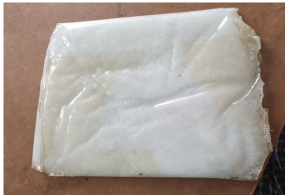
Fig-2: Unstitched orientation of fiber glass Reinforced Epoxy Composite
