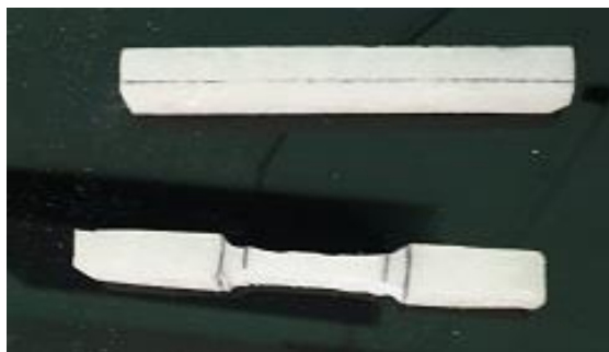
Specimens for tensile test and bending test
