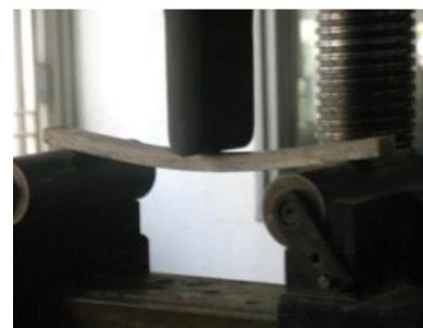
Fig -3: Flexural test arrangement
