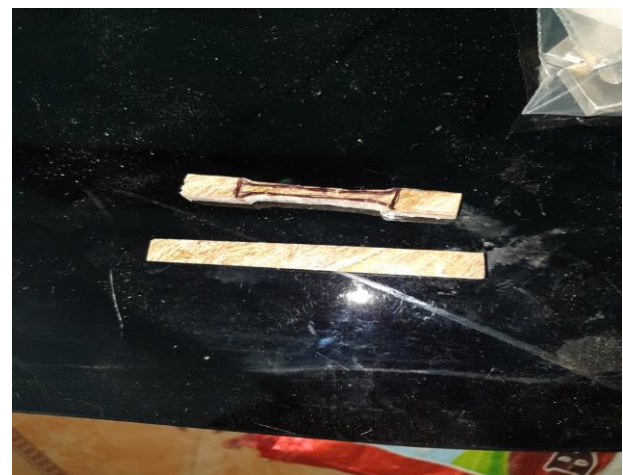
Fig-7: Specimen for tensile and bending stress.
