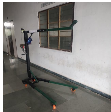
Photo 7: Portable Hydraulic Crane
