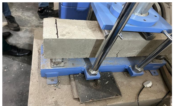
Figure 11. Failure of B2 beam
