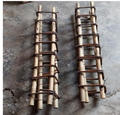
Figure 2. Bamboo stick placement
