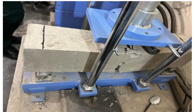
Figure 9. Failure of S beam
