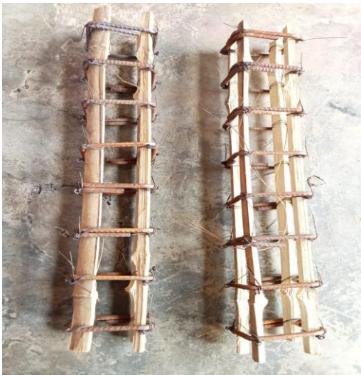
Figure 4. Laminated bamboo reinforcement
