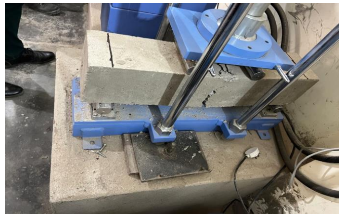
Figure 10. Failure of B1 beam
