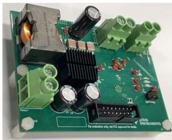
Fig. B. MPPT Solar Charge Controller
