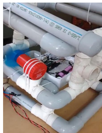
Figure 6: Installing bilge pump to the structure
