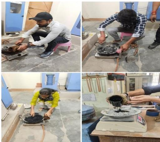
Mixing of Plastic, Aggregate and Bitumen
