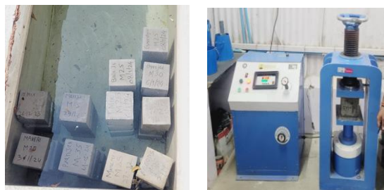
Figure 1 Casting and testing of cube.
