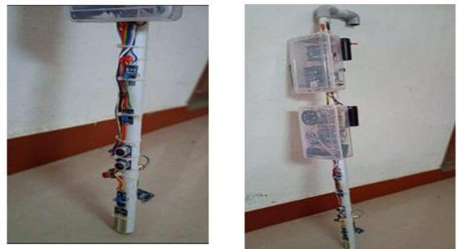
Fig. 2. Smart E-Stick with Electronic Circuitry and sensors
