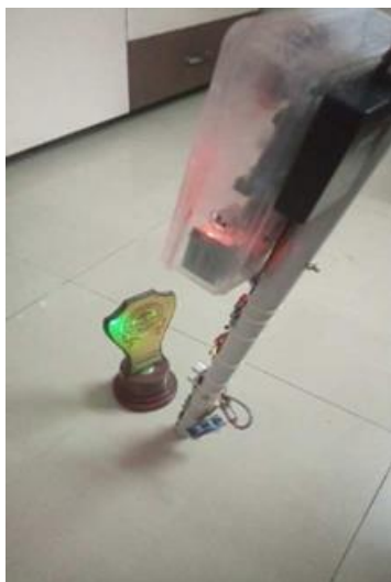
Fig.3. Detection of low level obstacle in Smart E-Stick
