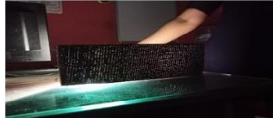
Fig 3.6 : Finished concrete block transmitting light
