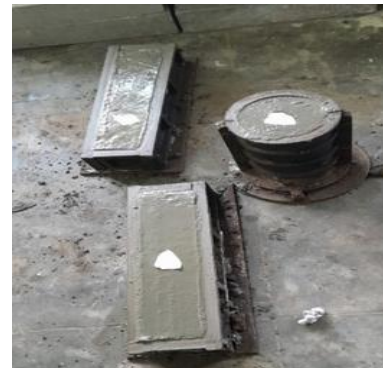
Fig 3.3 casting of specimens
