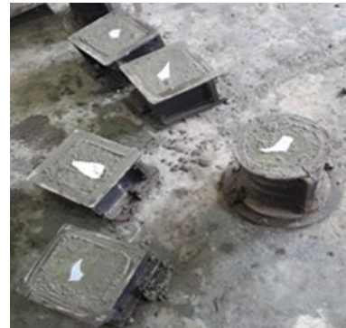
Fig 3.2 moulds for casting
