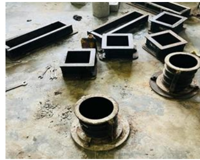
Fig 3.2 moulds for casting
